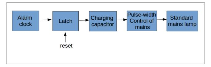
The use of a standard battery-powered alarm clock deals with points 2 and 3, and using a digital one rather than a clockwork one also deals with point 4. Travel alarms are also easy to obtain from my local household hardware shop. The idea of using the rising voltage on a slowly charging capacitor as a brightness control allows the use of 'junk box' components with no need for micro-controllers. The idea of using the existing mains lamp keeps everything simple and avoids extra clutter.
