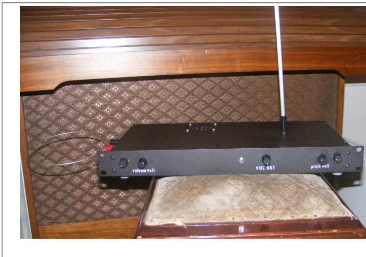
Fig 4.3.1: the finished instrument, built into a 19" rack cabinet. It is placed on an organ stool for photography, but would be played in open space.
